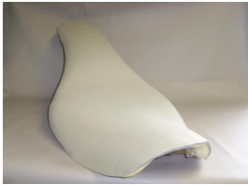
Use your contact adhesive again to glue the smoothing foam on. You will be covering the entire seat with the smoothing foam, not just the insertion area. The smoothing foam will help smooth the transition from insertion area to original seat foam. Stretch the smoothing foam when needed to avoid making wrinkles that will show under the seat cover. Trim off the excess smoothing foam that is hanging past the seat pan.
