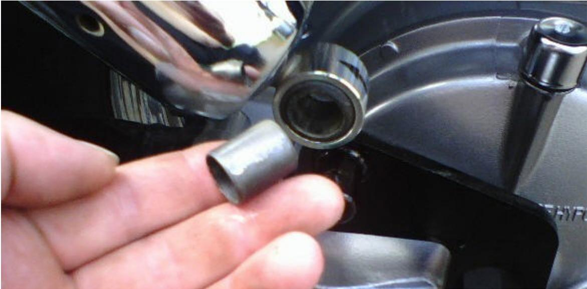
Apply some Loctite to the factory bolt and reinstall it. Loosen the upper shock bolt and use the pry bar to lift up on the wheel to attach the shock.
