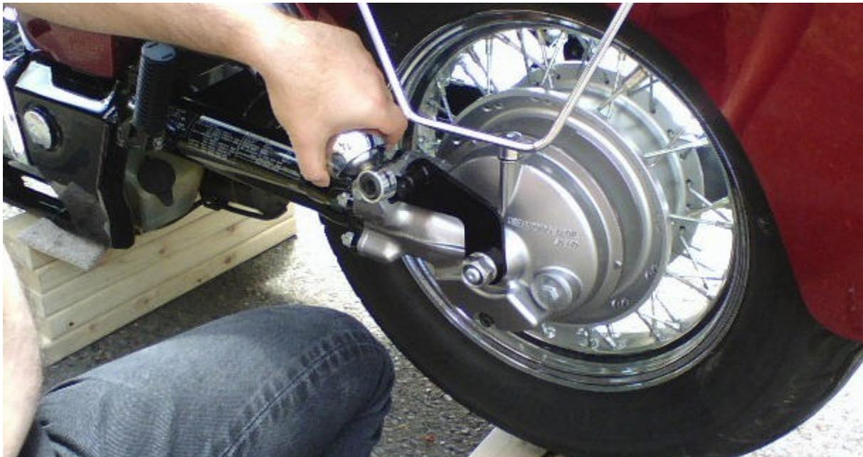
Now take the washers and bolts that came with your kit, apply a little Loctite and install into the NEW shock mounts.
