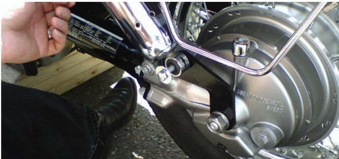
Last step: Tighten all 6 shock bolts (upper, old and new lower) along with the axel nut. Lower the bike off the jack, Torque everything to factory or instruction specifications.
