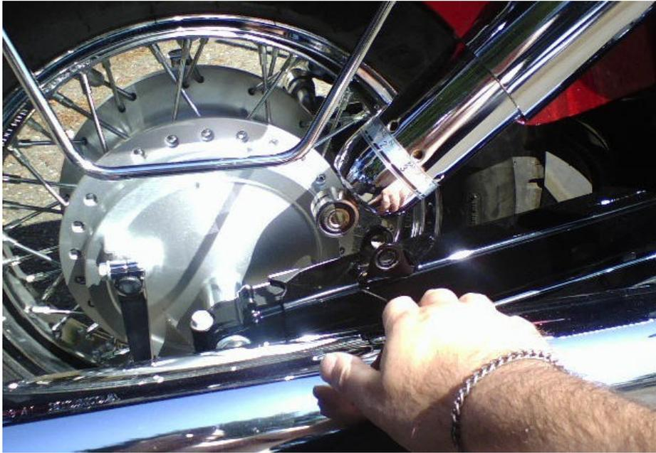
Take the LH assembly, (the smaller one) and slip it in the original shock mount. Apply some Loctite to the factory bolt and reinstall it *snug* not tight. Then remove the metal sleeve from the lower shock eye.
