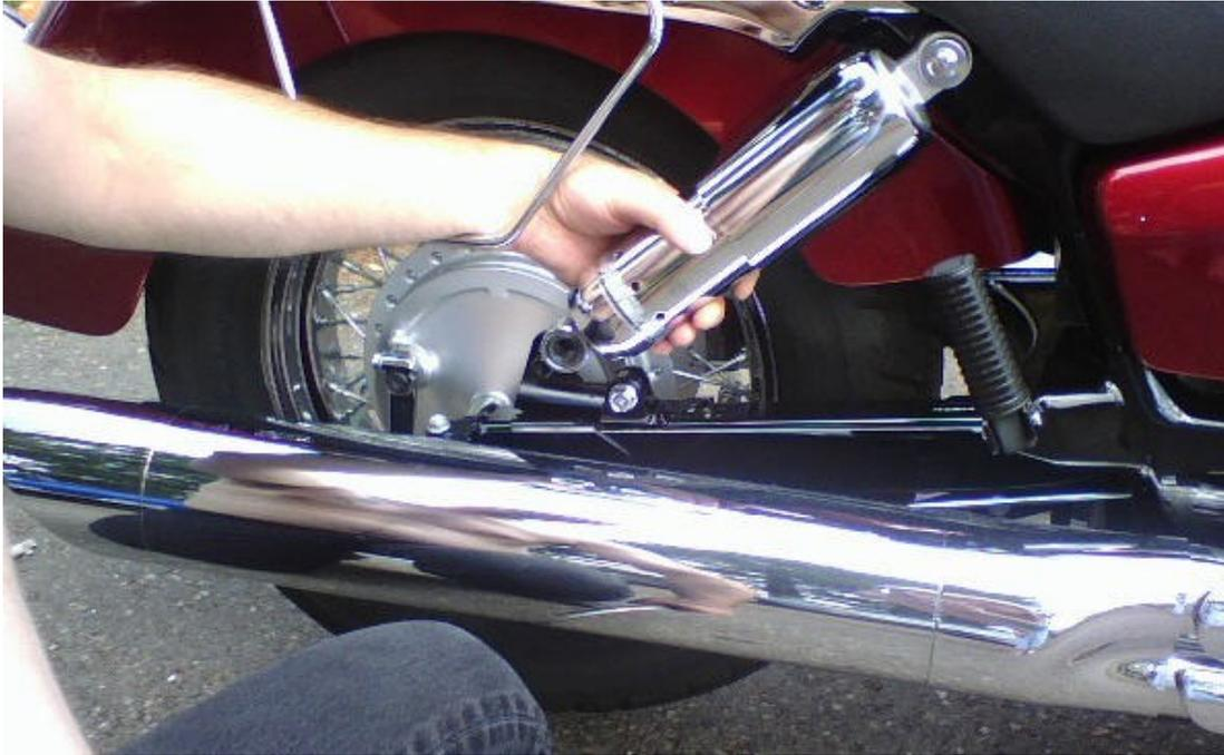
Move to the other side and remove the lower shock bolt,
